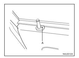
The security light (A) will flash once every 0.8 seconds to indicate that the theft-deterrent system is armed. The security light is located on the driver's door lock.
